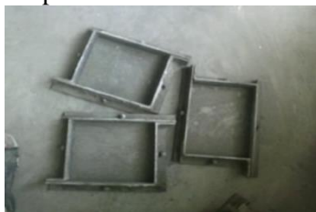
Figure.1. Moulds used for casting of paving blocks
