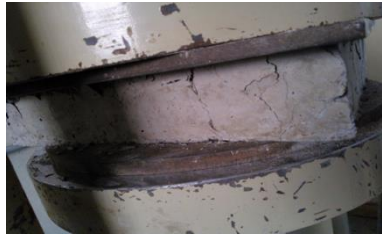
Figure.2. Paving block under compressive testing
